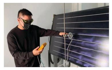
Solar radiation measurements in analyzing the characteristic performance of a solar collector with varying irradiance levels.
