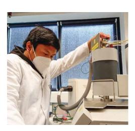
Set-up preparation for the synthesis of titanium carbohydrides (TiCH) powders under this multifunctional furnace system.
