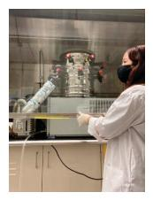
Freeze-drying of synthesized polymers.
