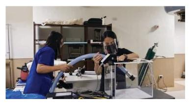
Setting up a radiotherapy water phantom used for quality assurance of a medical linear accelerator
