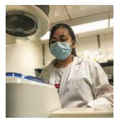
Performing lysis of cells by adding lysis buffer and glass beads into the solution and placing it in a homogenizer which will break open the cells to release the DNA.
